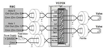
Fuse 24Vdc input with 5A maximum, UL-listed, fast-blow fuse. One fuse suffices for up to 10 VC2124s. For maximum protection, use one 500mA fuse per VC2124.
