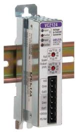
The VC2124 voltage-to-current converter transforms ±10V signals into current signals capable of driving hydraulic servo valves or similar loads. It also provides a convenient way to set the full scale current to match valve requirements, limit maximum current, or set optimum working ranges.
